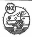
Don't drive over your tank or any buried components in your system, unless they've been equipped with a special traffic lid. If the system is subject to possible traffic, put up a barricade or a row of shrubs.
